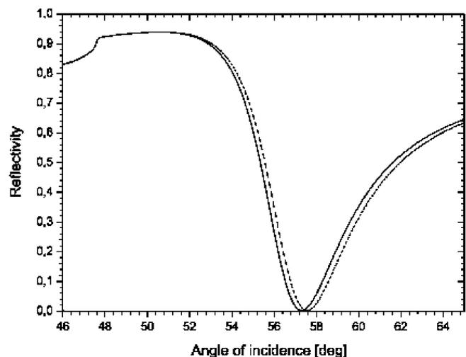
Fig. 2. The reflectivity before and after protein adsorption ( $90^\circ$  prism with  $n = 1.84$ , gold:  $\varepsilon = -12.5 + i1.5$  and  $t = 45$  nm, protein:  $n = 1.42$  and  $t = 2.5$  nm, water  $n = 1.333$ ,  $\lambda = 633$  nm). The adsorption leads to a shift of the plasmon resonance  $\theta_0$  which is the essential parameter of an SPR curve.
