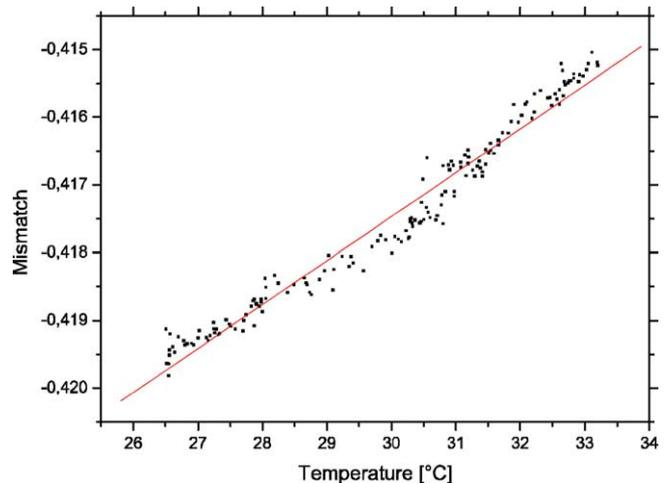
Fig. 10. Measurement of the mismatch  $M$  as a function of the temperature of the air. The smallest detectable change of the refractive index of the analyte can be estimated to be in the order of  $10^{-7}$ .
