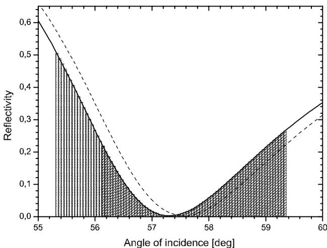
Fig. 6. Illustration of the mismatch concept using a goniometer setting  $\theta_0$  and an angular range of  $\delta\phi = 2.0^\circ$ . The vertically striped area matches the diagonal striped area and the mismatch  $M$  vanishes. All settings are then kept fixed and a mismatch is observed as a consequence of the adsorption. The solid line refers to the reflectivity before and the dashed one after adsorption.
