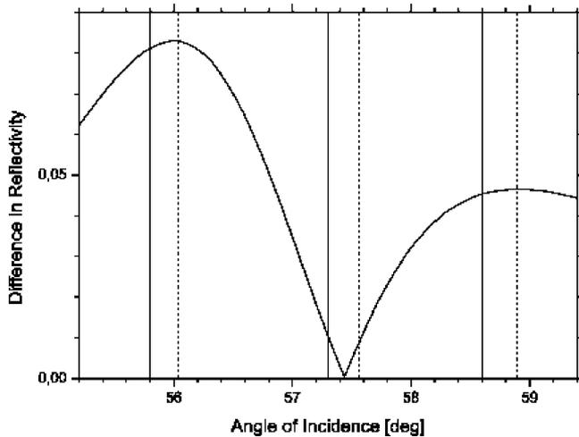
Fig. 3. Difference in the reflectivity before  $R_0$  and after protein adsorption  $R_f$  as a function of the angle of incidence. The solid vertical line refers to the point of inflection, reflectivity minimum and second point of inflection of the reflectivity scan before (solid) and after adsorption (dashed). Due to the asymmetry of the SPR curve the best choice is the point of inflection at lower angles.
