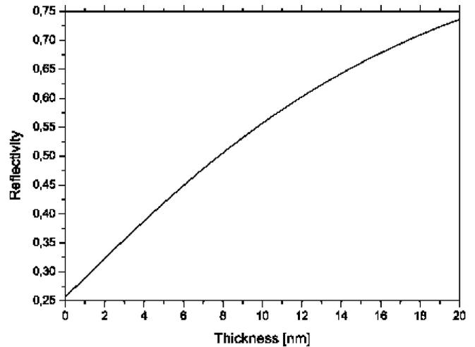
Fig. 4. Dependence of the reflectivity as a function of the layer thickness for a fixed setting of the refractive index  $n = 1.4$ . The angle of incidence  $\Theta$  matches the point of inflection at lower angles. The reflectivity increases in a monotonous fashion and a direct proportionality holds for a layer thickness up to 10 nm.
